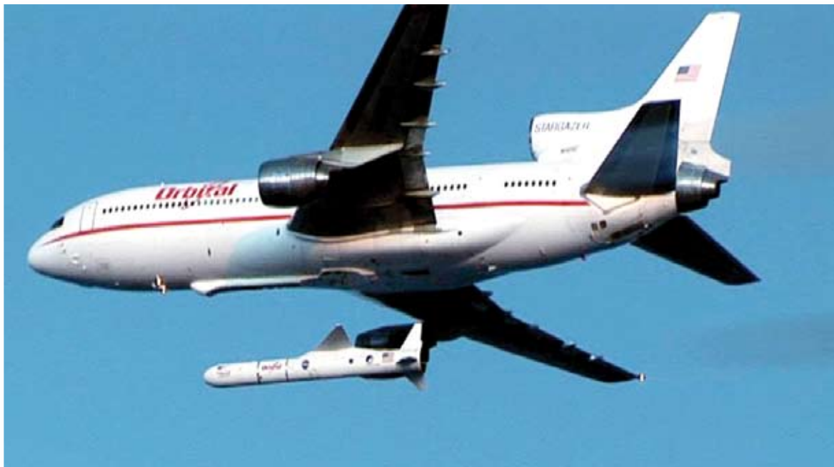
(above) The Orbital Sciences L-1011 jet aircraft releases the Pegasus XL launch vehicle carrying the Space Technology 5 spacecraft with its trio of micro-satellites from Vandenberg Air Force Base, Calif., on March 22, 2006.
