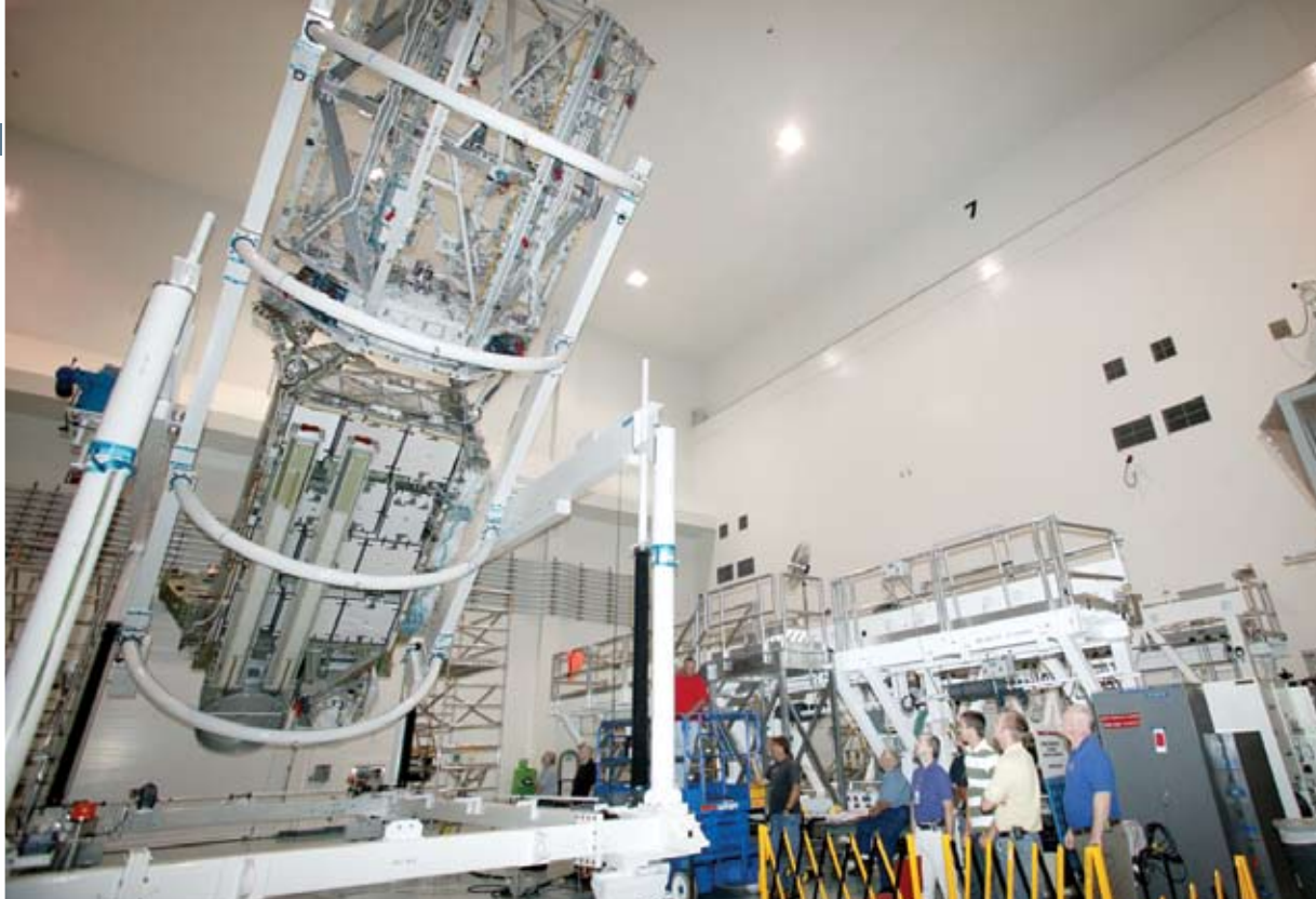
The S3/S4 truss segment is tilted on a work stand inside the Space Station Processing Facility high bay during processing to prepare the element for delivery to the space station on mission STS-117.
