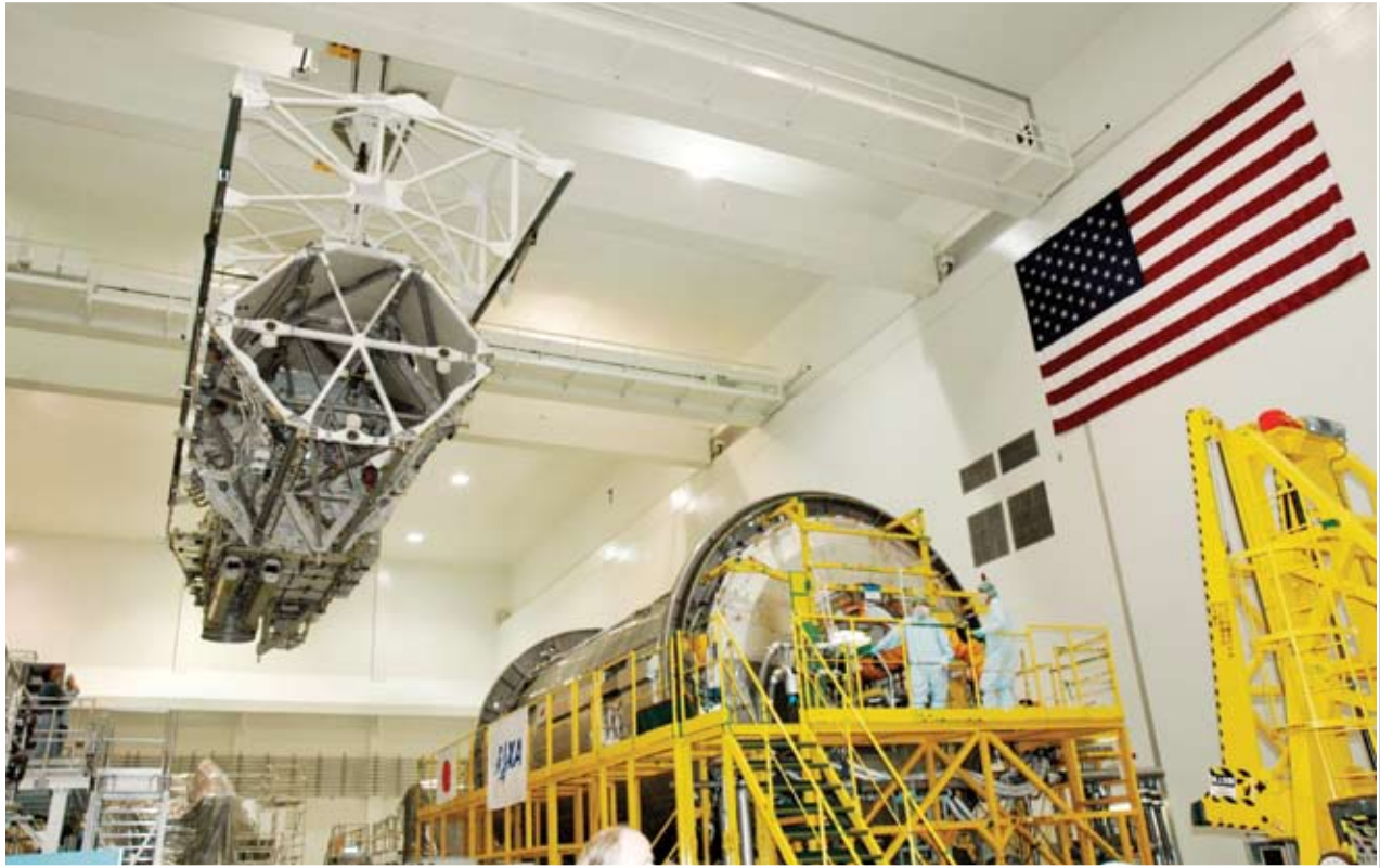
An overhead crane moves the P3/P4 truss segment across the floor to the waiting payload canister inside the Space Station Processing Facility. The truss was delivered to the space station on mission STS-115.
