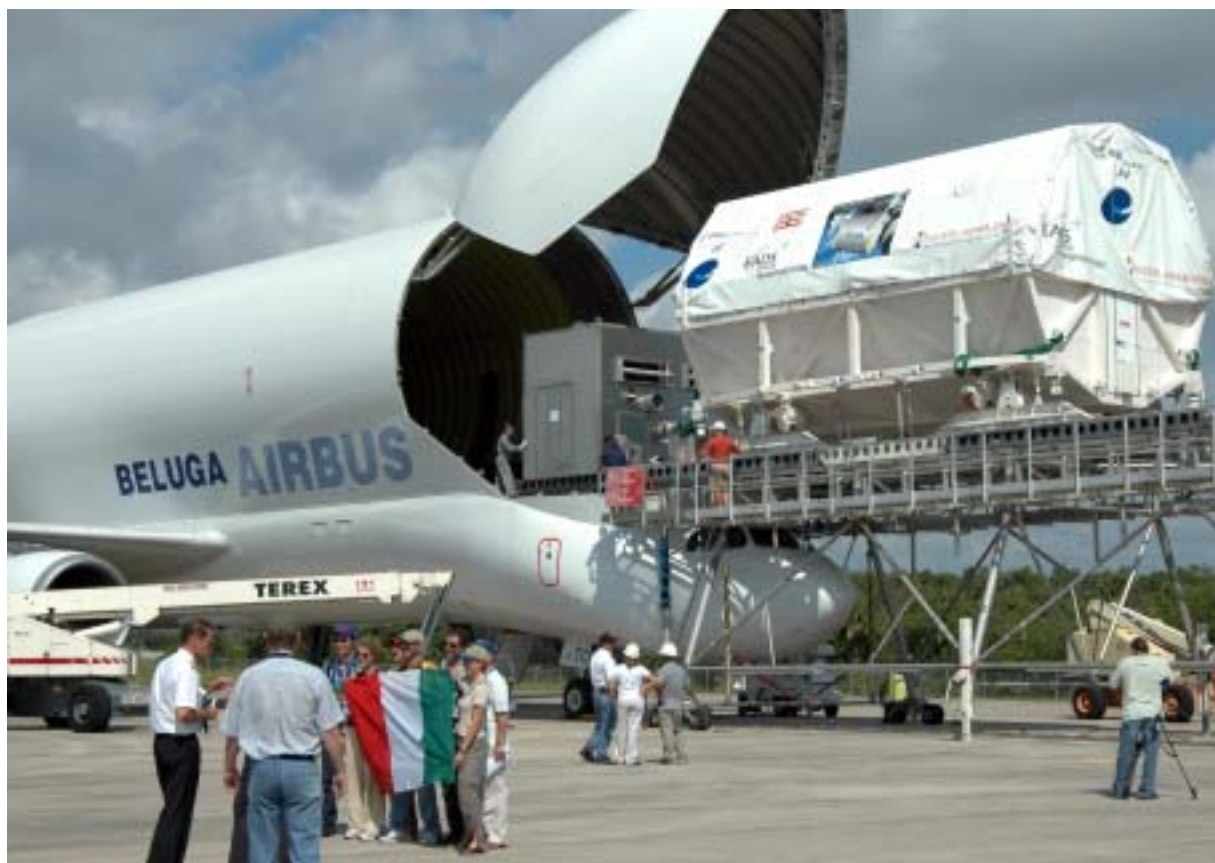
THE EUROPEAN Space Agency's research laboratory, Columbus, is offloaded from a Beluga aircraft onto a platform before being lifted onto a flatbed truck and transported to the Space Station Processing Facility.
