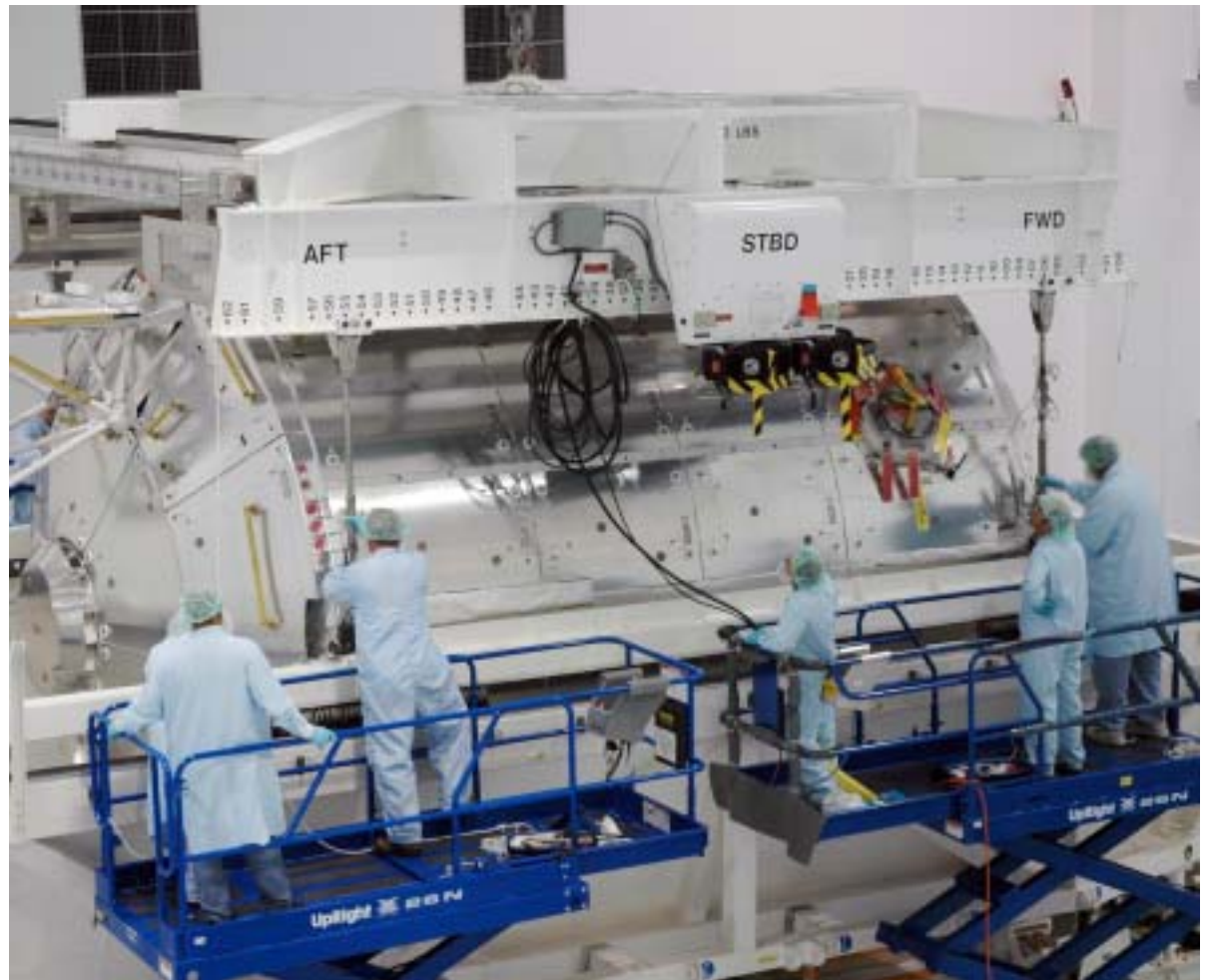
INSIDE THE Space Station Processing Facility, an overhead crane is lowered onto the Columbus module to lift it out of its transportation canister.
