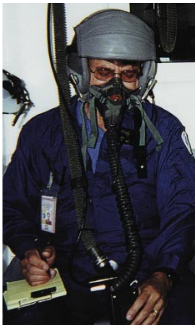
Jan Zysko, chief of the data and electronic systems branch of KSC's Spaceport Engineering and Technology directorate, tests the Personal Cabin Pressure Altitude Monitor in an altitude chamber at Tyndall Air Force Base in Florida. Zysko invented the pager-sized monitor that alerts wearers of a potentially dangerous or deteriorating cabin pressure altitude condition.
