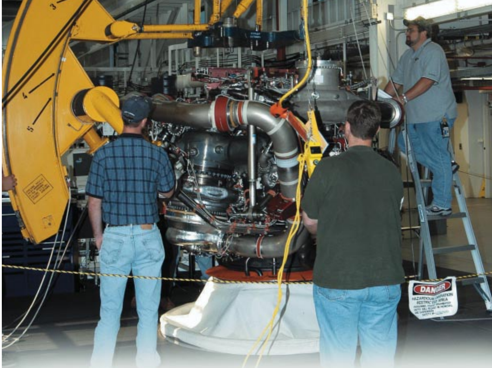
Inside the Space Shuttle Main Engine Processing Facility, Boeing-Rocketdyne technicians prepare to move the first main engine fully assembled at KSC. Workers prepare to place a sling around the engine to assist its lift from a vertical work stand into a horizontal position in preparation for shipment to NASA's Stennis Space Center in Mississippi to undergo a hot-fire acceptance test.
