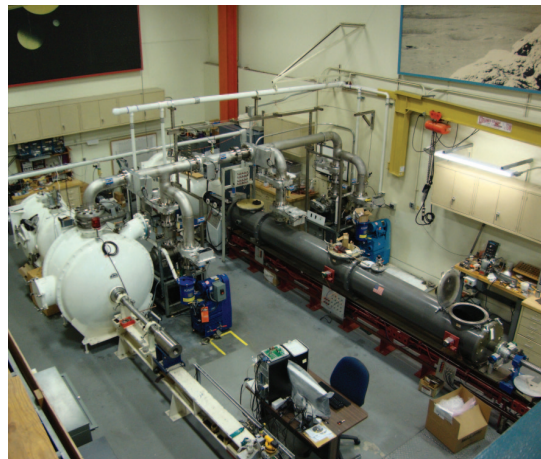
Overhead view of the 5 mm Light-Gas Gun (right) and Flat-Plate Accelerator (white, left) in the Experimental Impact Laboratory at the Johnson Space Center.
