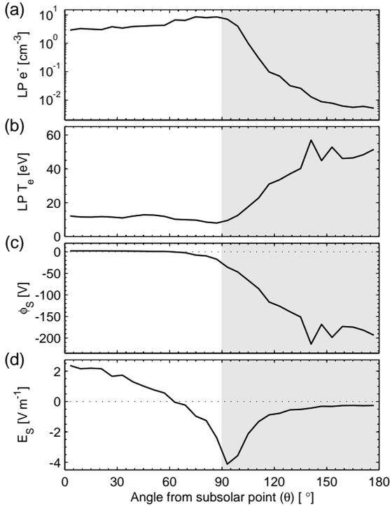
Figure 3. Lunar surface charging predictions based on LP/ER data in the solar wind. Shown are observations of (a) electron concentration,  $n_e$  ( $\text{cm}^{-3}$ ) and (b) electron Maxwellian temperature,  $T_e$  (eV); and predictions for (c) surface potential,  $\phi_S$  and (d) electric field,  $E_S$ .
