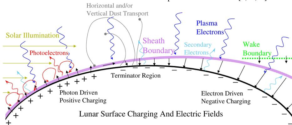
Figure 1. Schematic of the lunar electrostatic environment in the solar wind (not to scale).
