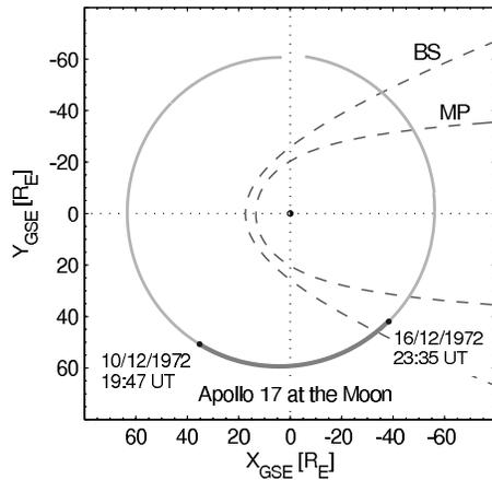
Figure 4. The Moon's orbit about the Earth during the Apollo 17 mission. View is from above the north pole with the Sun to the left. Also shown are empirical models of the Earth's bow shock, BS, and magnetopause, MP, boundaries.
