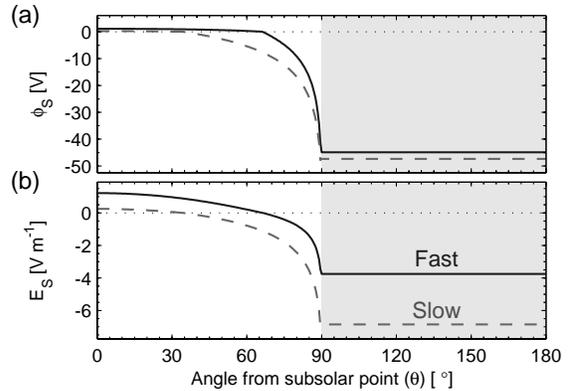
Figure 2. Lunar surface charging predictions for typical fast and slow stream solar wind conditions. Shown are (a) surface potentials,  $\phi_s$  (V), and (b) electric fields,  $E_s$  ( $\text{V m}^{-1}$ ). The grey shading indicates the lunar nightside.
