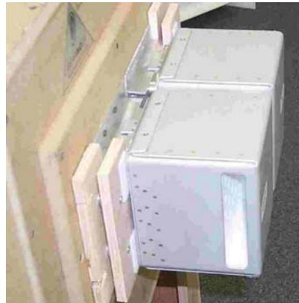
Figure 5: CGBA muffer attached to test fixture
