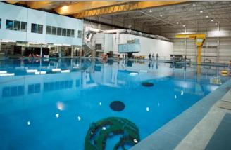
(20 ft above ground level and 20 ft below) and holds 6.2 million gallons of water. Even at this size, the International Space Station, at 350 ft x 240 ft when complete, will not fit inside the NBL.
