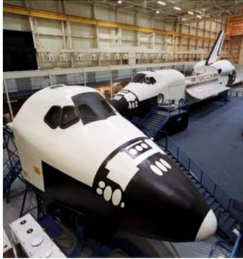
The Integrated Training Facility at JSC is where astronauts learn how to fly the shuttle and receive training in station programs. The shuttle side houses simulators that test the skills of flight crews and ground controllers for all phases of a shuttle mission. The station side provides mission training, flight procedures verification and contingency mission support for the Space Station Program.
