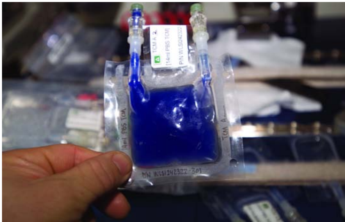
View of a Tissue Culture Module as part of Fluid Dynamics Investigation for the Cellular Biotechnology Operations Support System experiment flown during Expedition 8.
