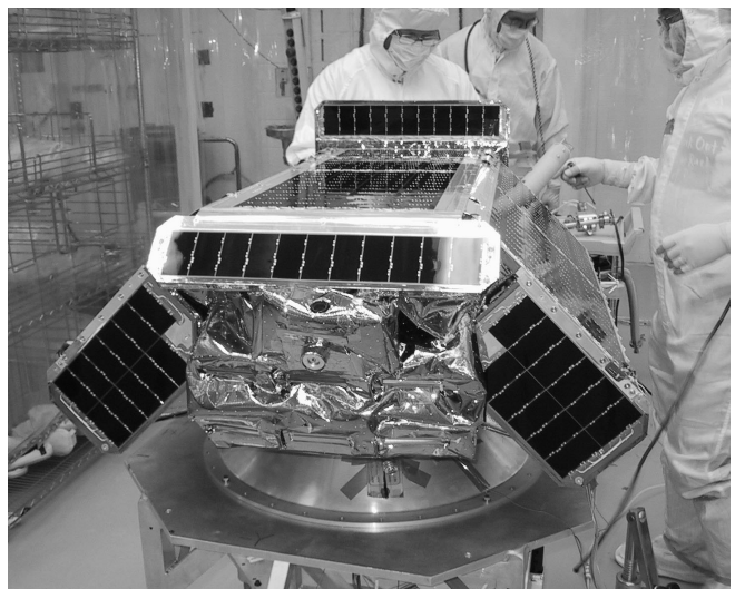
CHIPS six apertures for observing the ISM are located just below the small disk in the center of the forward end. The black rectangles are solar cells. (Photo UCB)
