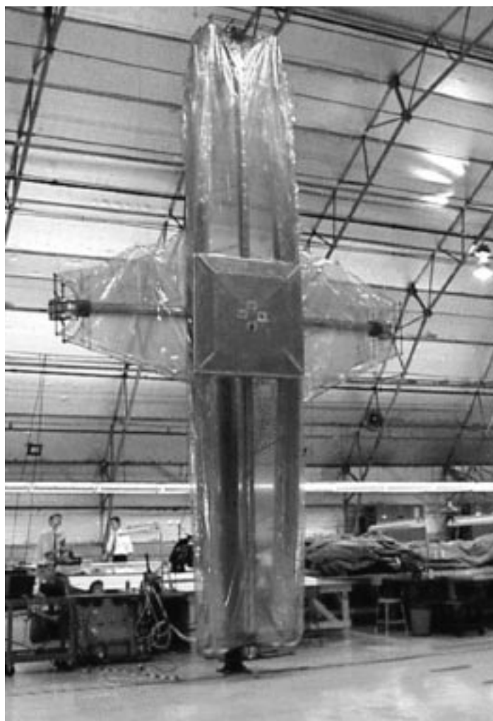
Engineers perform tests on a model of the NGST inflatable sunshield.
