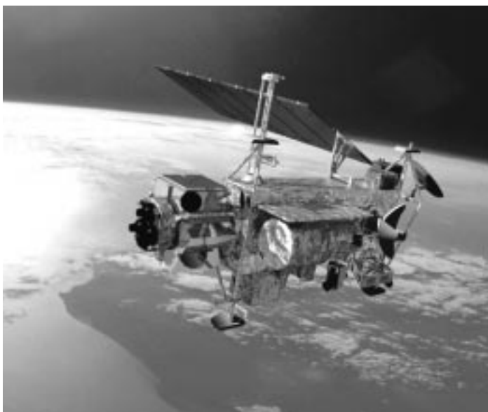
Deployed from the Shuttle on September 15, 1991, the Upper Atmosphere Research Satellite, depicted in this artist concept, was able to map chlorine monoxide, an ozone-destroying radical, within the Arctic vortex.
