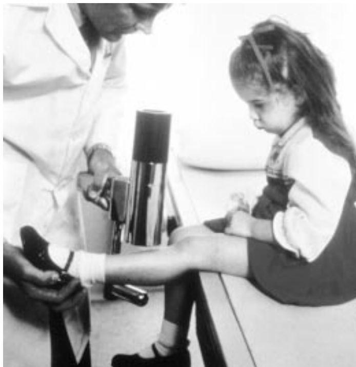
The Goddard-developed Lixiscope produces an instant image through use of a small amount of radioactive isotope.
