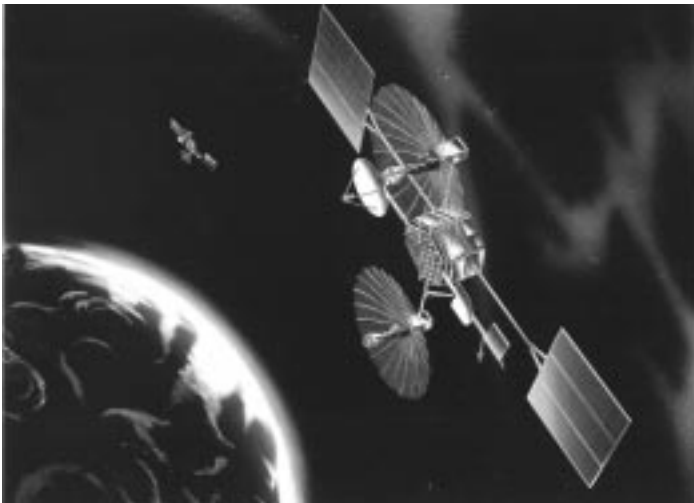
Six Tracking and Data Relay Satellites, like these shown in this drawing, provide NASA's primary communication link with the Space Shuttle, International Space Station and satellites in low-Earth orbit.
