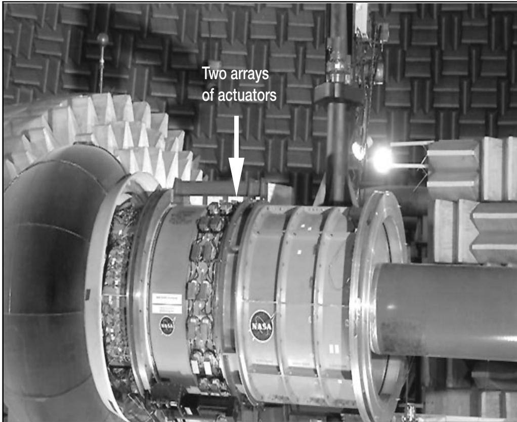
*The Active Noise Control Fan at NASA Glenn showing two circumferential arrays of acoustic actuators.*
