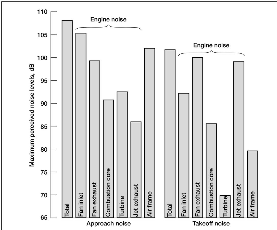
A breakdown of the noise components of a typical engine with 1992-level technology during takeoff and approach to landing indicates the large part played by engine noise. Note: because decibels are logarithmic values, the graph's total bar is the sum of the individual bars.
