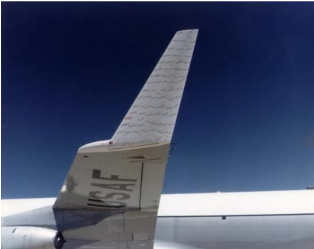
Close-up of winglet on KC-135 test aircraft, with attached tufts displaying flow of air over winglet surface. NASA Photo EC79-11481
