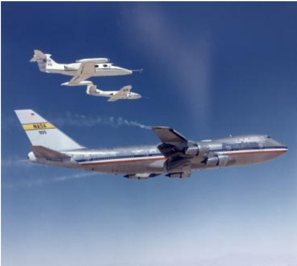
A Learjet and an Air Force T-37 meet in the skies over NASA Dryden for a series of flights to study the hazards of wake vortex generated by large aircraft. Studies conducted from the late 1960s to 1974 used large aircraft as wake generators and smaller instrumented aircraft such as the Learjet and T-37 were flown into the vortices to determine vortex strength and safe separation distances. The 747 is the same one acquired by NASA and later modified to carry space shuttles.
