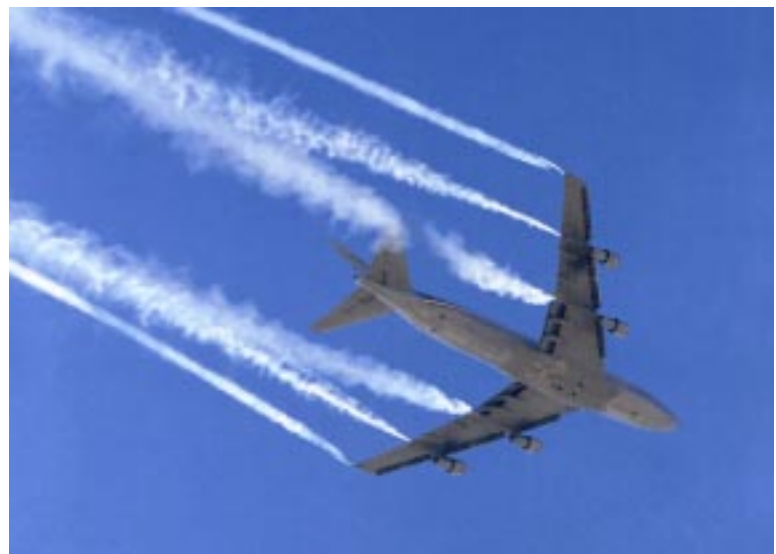
Smoke streams from on-board generators of a 747 jumbo jet to present a visual picture of the magnitude of wake vortices created by large aircraft. This 747 is the same one acquired by NASA and later modified to carry space shuttles.
