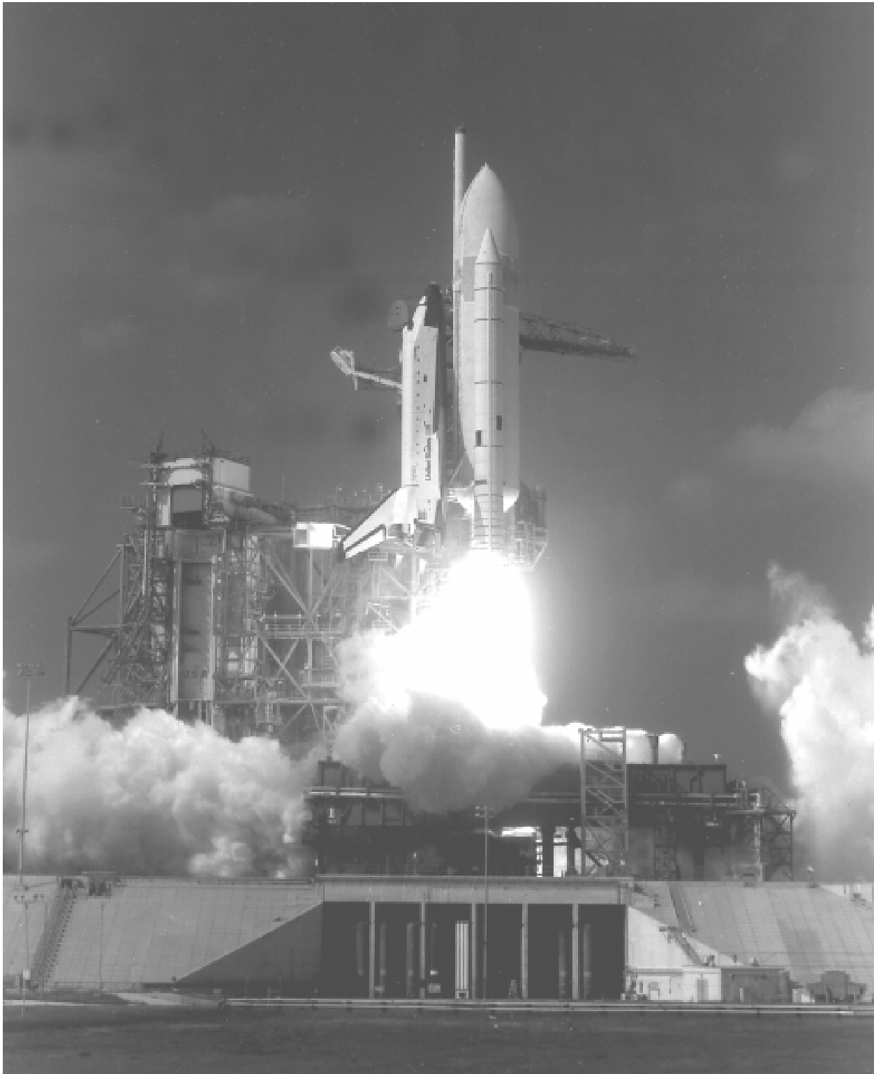
Figure 3. Space Shuttle Columbia climbs skyward on its second mission into space from NASA's Kennedy Space Center, Florida, on November 12, 1981. This photograph shows one of the two giant solid rocket boosters firing to provide the lion's share of the orbiter's lift for the first 24 nmi of ascent into space.
