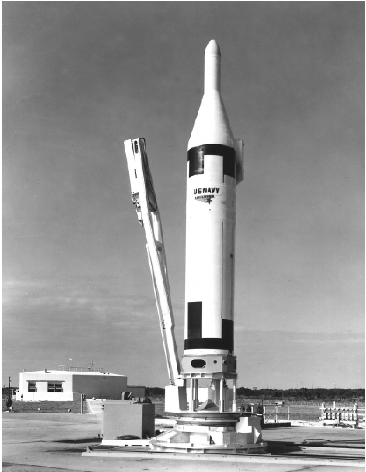
Figure 1. A Polaris A2X test missile on the launch pad at the Atlantic Missile Test Range, Cape Canaveral, Florida. The A2X is the prototype for the 1500-nmi Polaris A2 missile that became operational in 1962.
