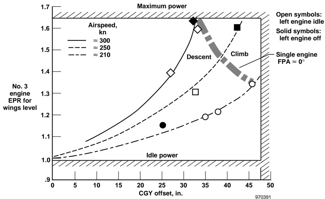
Figure 15. Effect of *CGY* offset on EPR on the number 3 engine required for wings-level flight, MD-11 FDS, flaps and slats up, gear up, an altitude of approximately 10,000 ft, gross weight approximately 400,000 lbm, center engine at idle power.
