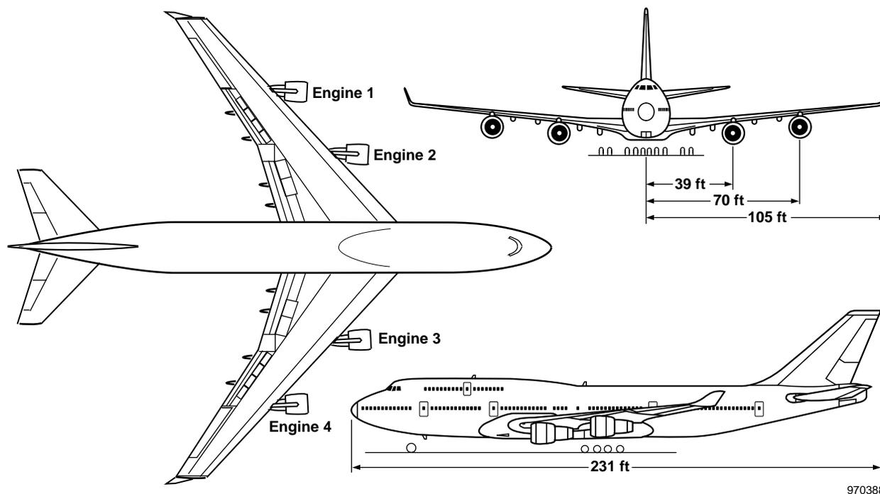
Figure 9. Three-view drawing of the B-747-400 airplane.
