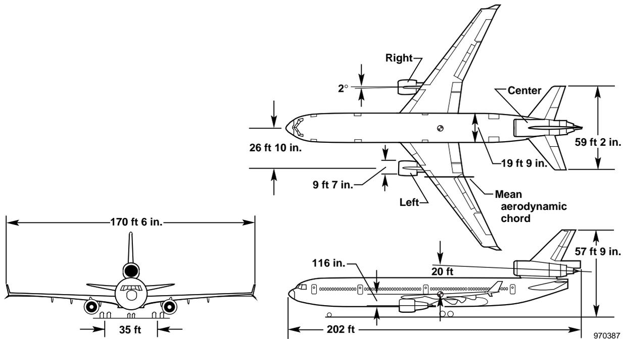
Figure 8. Three-view drawing of the MD-11 airplane.
