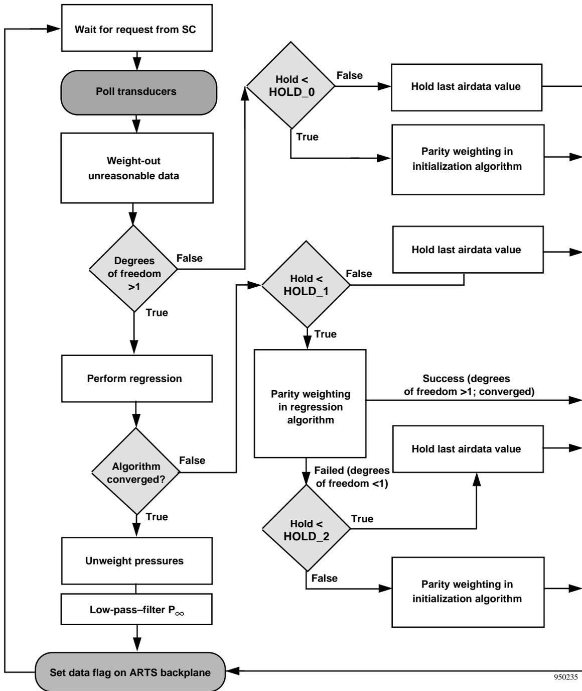
Figure 6. Fault-tolerant data flow through RT-FADS computational cycle.
