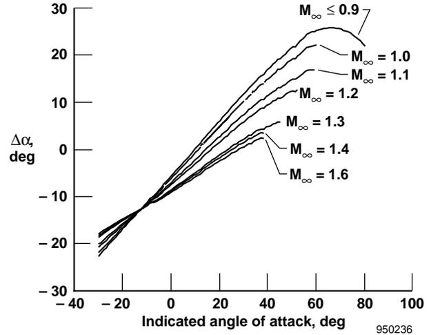
Figure 7. RT-FADS upwash calibration curve.
