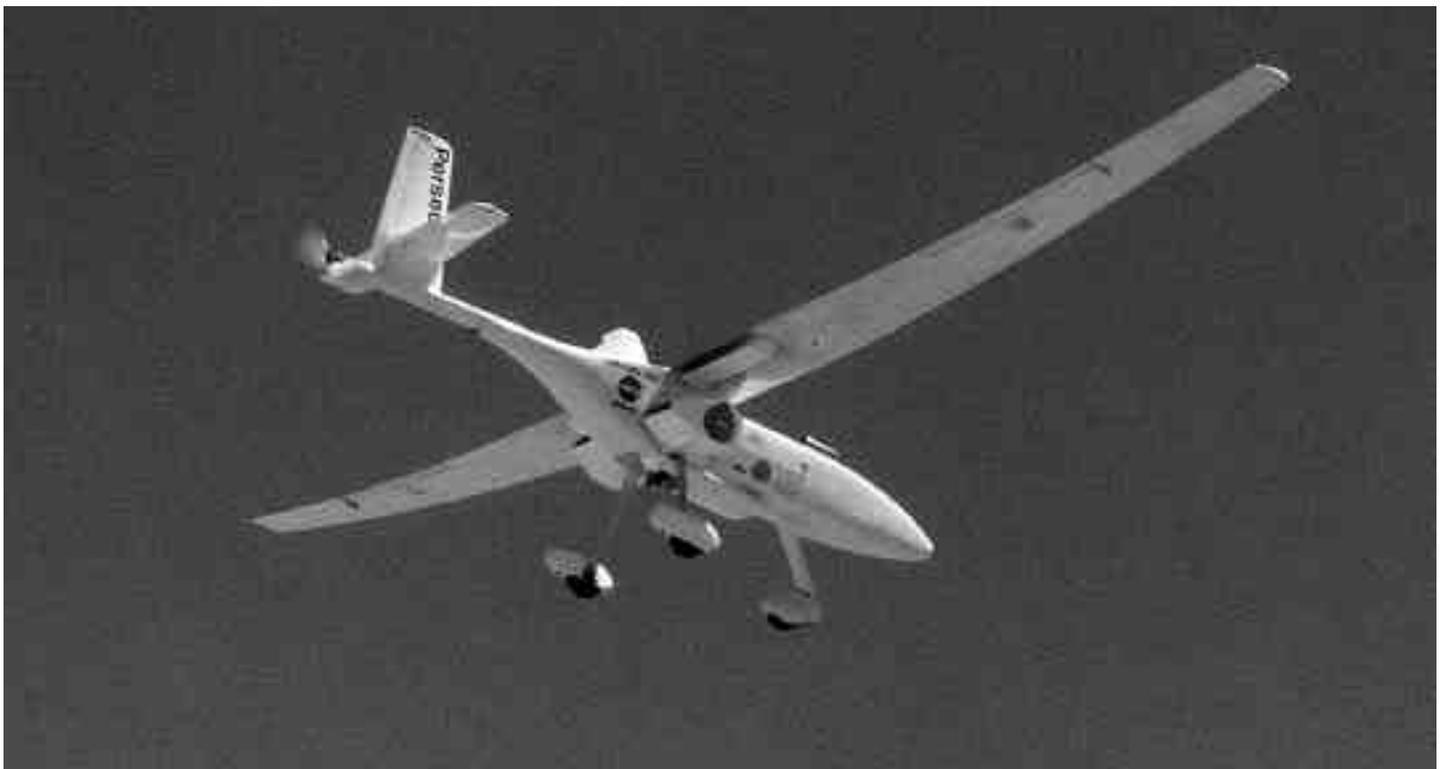
The Perseus B is a remotely piloted aircraft developed as a design and performance testbed under NASA's Environmental Research Aircraft and Sensor Technology (ERAST) project.
