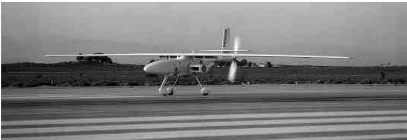
71.5 feet to enhance high-altitude performance—the Perseus B returned to Dryden in the spring of 1998 for a series of four flights. Those flights culminated with a flight on June 27 to an altitude of 60,280 feet, establishing an unofficial altitude record for a single-engine, propeller-driven remotely piloted aircraft.
