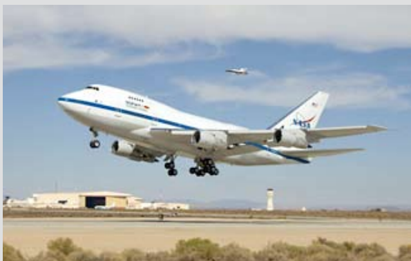
NASA photo by Tony Landis NASA's Stratospheric Observatory for Infrared Astronomy, SOFIA, lifted off from Edwards Air Force Base at mid-day Oct. 11, 2008, on the first in a series of flight tests intended to verify the flight performance of the highly modified Boeing 747SP to its design capability.
