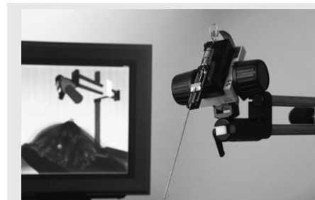
The Ames Smart Systems Research Lab team was a recent recipient of the Space Act Award for their Smart Surgical Probe (above). The probe provides intelligent fusion of data from various sources that provides accurate diagnosis from tissue samples.
