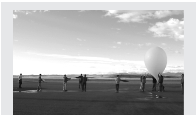
The Reentry Breakup Recorder (REBR) balloon ready for launch. Preston Partridge, second from left, holds the REBR capsule. REBR is designed to provide detailed information on how an upperstage or spacecraft breaks apart during reentry.
