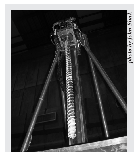
The Mars drill prototype device at NASA Ames is controlled by artificial intelligence. Such a device was used in the Arctic in July to evaluate the automation software, in preparation for its future use on Mars.
