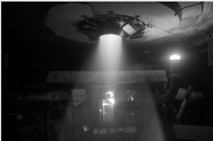
Arc jet test at the NASA Ames Interaction Heating Facility (IHF) (top view) with thermal protection system (TPS) material coupon glowing after test completion. The tests are a critical part of developing new TPS materials.
