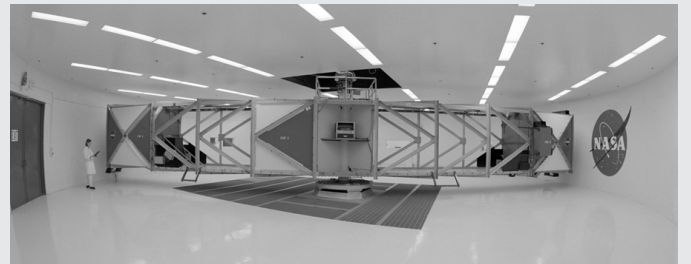
The 20-G centrifuge at NASA Ames is a machine that creates artificial gravity forces by spinning and that can simulate up to 20 times the normal forces of gravity we experience on Earth.
