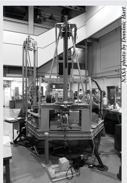
The 'Mars Drill' at Ames (above) brings subterranean 'core' samples to the surface that are 10 inches (25 centimeters) long and one inch in diameter (2.5 centimeters) while operating with low power and no drilling fluids. An automated core-and-sample handling facility extracts the cores from the drill, passing them to a suite of instruments on a 'Mars lander platform' for analysis.
