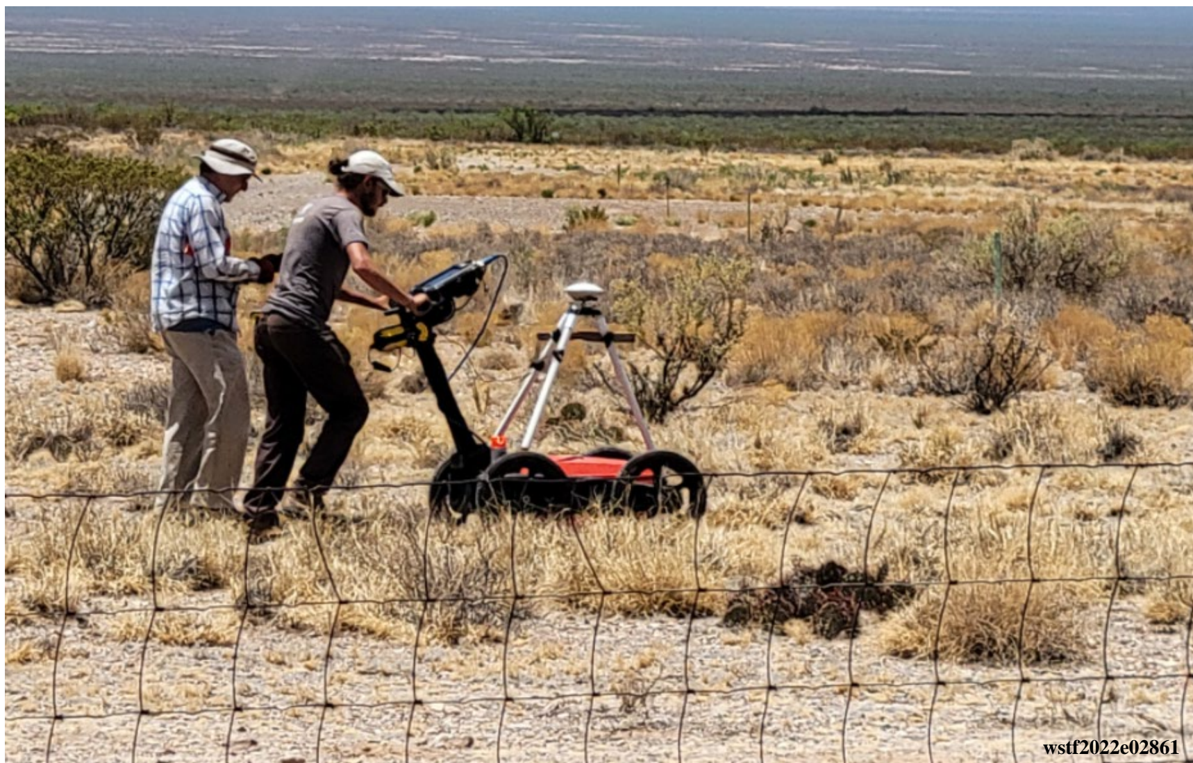
GPR suitability test and data recording on the 700 Area Landfill cap (view to the west [May 28-29, 2021]).
