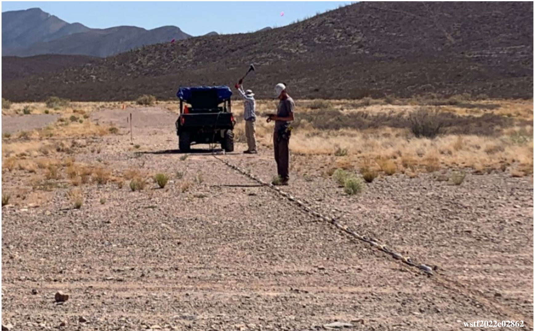
AMASW survey line, energy source, and data recording on the 700 Area Landfill cap (view to the northwest [May 28-June 9, 2021]).
