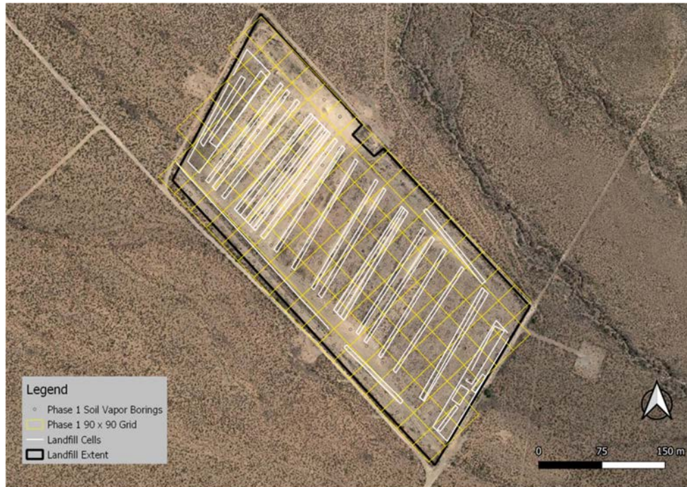
Figure 2. Detail of the Area 700 Landfill, in black rectangle, at approximately 25 acres. Also shown are the 90 x 90 foot grid (yellow lines), soil vapor borings (black circles), and approximate extent of landfill trench cells (white) (aerial photography courtesy of Google Earth Images).
