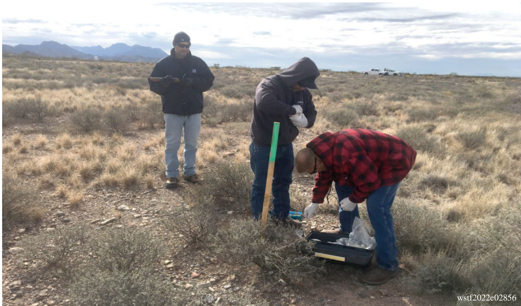
Shallow SVS sample module deployment and data recording at a staked sampling node on the 700 Area Landfill cap (view to the south [November 25-December 1, 2019]).
