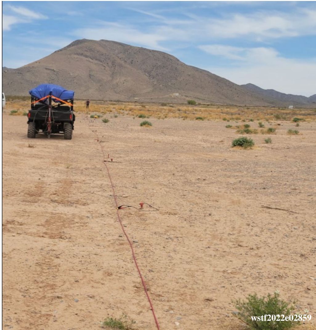
Enhanced passive seismic survey line with geophones and field support vehicle on 700 Area Landfill cap (view to the northwest [May 25-27, 2021]).
