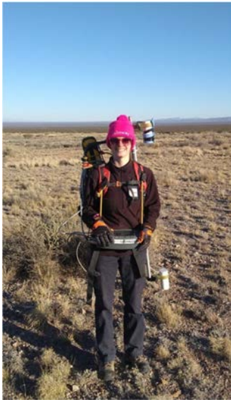
Photo 3. Geometrics G-858, in vertical magnetic gradiometry mode in a backpack configuration.
