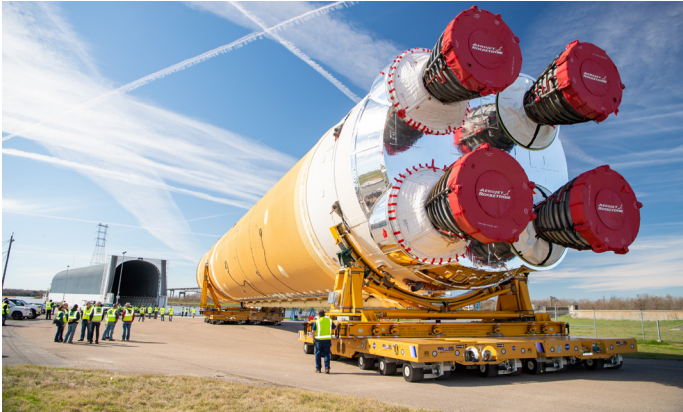
Crews moved the flight hardware for the first Artemis mission to NASA’s Pegasus barge on Jan. 8 in preparation for the core stage Green Run test series at NASA’s Stennis Space Center near Bay St. Louis, Mississippi. (NASA/MSFC/MAF)
