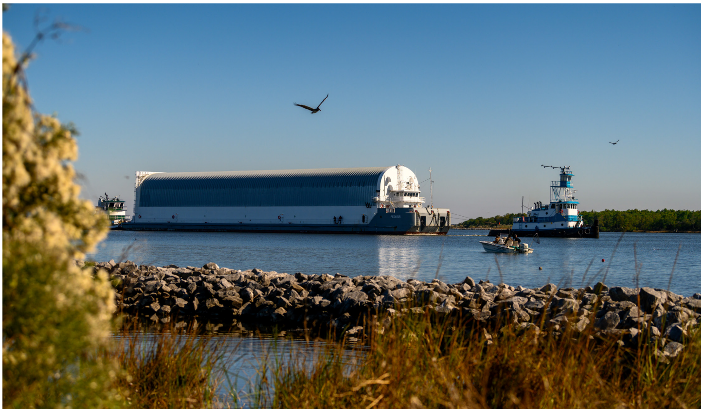
The Pegasus barge, originally used during the Space Shuttle Program, has been redesigned and extended to accommodate the SLS rocket's massive 212-foot-long core stage - the backbone of the rocket. (NASA/MSFC/MAF)
