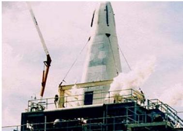
Test Stand 402 is an ambient test stand, capable of accommodating approximately 60 K lbf (270 kN) thrust engine, firing vertically downward into a water-cooled deflector. The system is 4885 ft above sea level and includes a maximum test article envelope of 15.5 ft by 15.5 ft by 30 ft (maximum with the stand enclosure in place). It has dual-position, vertical or horizontal firing capability, and portable tankage. This stand is currently mothballed.
