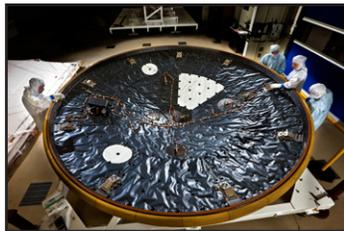
the heat shield during atmospheric entry and descent at Mars. MEDLI transmitted to Earth important engineering data concerning the atmospheric entry conditions and heat shield performance. The data is being used to refine the design of future heat shields, minimizing weight and improving performance. Infusion customers include NASA's Mars Exploration Program and NASA's Human Exploration and Operations Mission Directorate.
