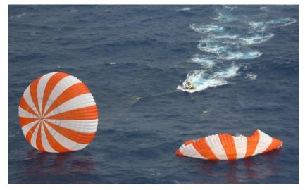
lose one of its main parachutes, the two remaining chutes would still permit a safe landing.
