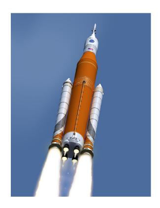
upper stage. The next planned evolution of the SLS, Block 1B, will use a new, more powerful Exploration Upper Stage (EUS) to enable more ambitious missions and deliver a 105-metric-ton (115-ton) lift capacity. A later evolution, Block 2, would replace the current five-segment boosters with a pair of advanced solid or liquid propellant boosters to provide a 130-metric-ton (143-ton) lift capacity. In each configuration, SLS
