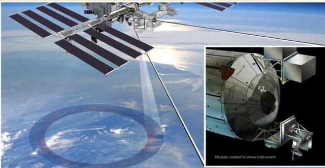
*This artist's rendering of the ISS-RapidScat instrument (inset), will measure ocean surface wind speed and direction and help improve weather forecasts, including hurricane monitoring. It will be installed on the end of the station's Columbus laboratory. (NASA/JPL-Caltech/Johnson Space Center)*
