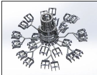
Fig. 6: Microspine gripper (JPL)
