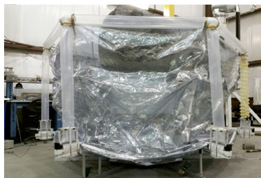
Fig. 5: Proof-of-concept inflatable asteroid capture system (JPL)
