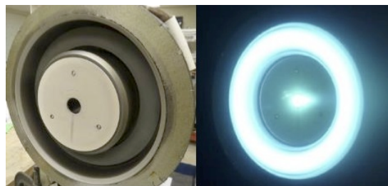
Fig. 3: GRC 300M Hall thruster
