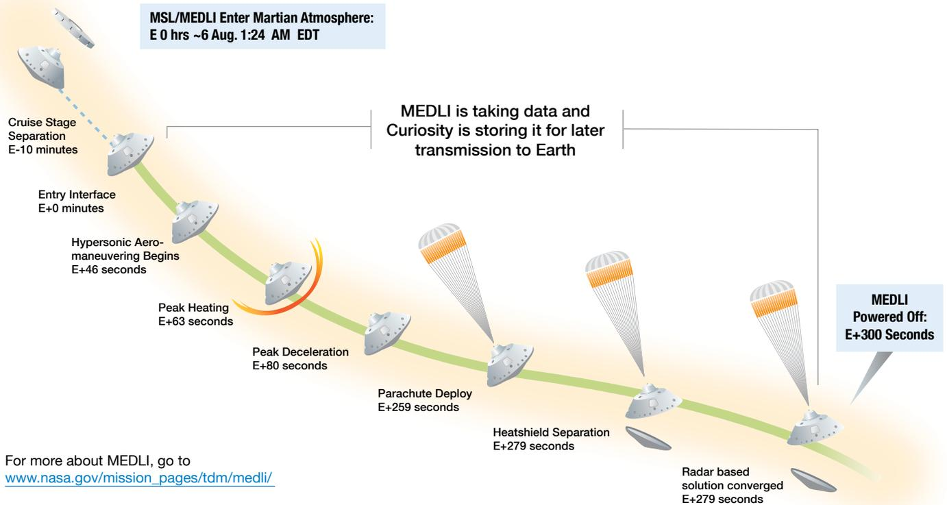
could withstand the heat of entry. The cross pattern allowed MEDLI engineers to determine the orientation of the MSL aeroshell and how it changed during the less than 10 minutes MSL took to fly from the top of the atmosphere to the surface. Engineers used this information to see how accurately computer models predicted the spacecraft's path and aerodynamics, as well as to determine the atmospheric density and winds it encountered.
