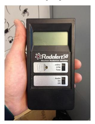
Figure 44 - Radalert50 Nuclear Radiation Monitor
