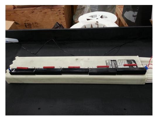
Figure 26 – 100kV diode bridge and test capacitor.
