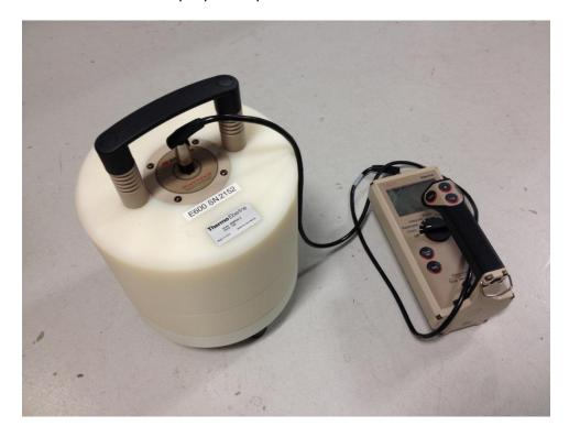
Figure 43 - Thermo Eberline SWENDI 2 neutron probe with counter.
