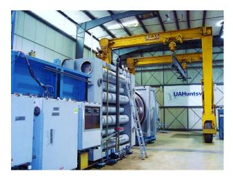
Figure 47 - The Charger 1 Pulse Power Research Facility provides 3 TW and 572 kJ of electrical energy into pinch loads.
