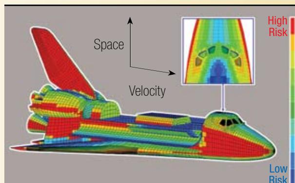
*Shuttle impact risk from orbital debris  $\geq 3\text{mm}$  diameter*
