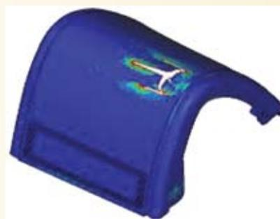
*NESC reviewed models for predicting damage to reinforced carbon-carbon and tile caused by foam and ice being shed from the external tank during ascent*
