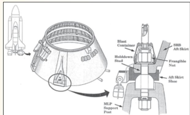
*The recurring anomalies review highlighted areas for additional program disposition, such as the solid rocket booster holddown post stud hang-up issue illustrated above*
