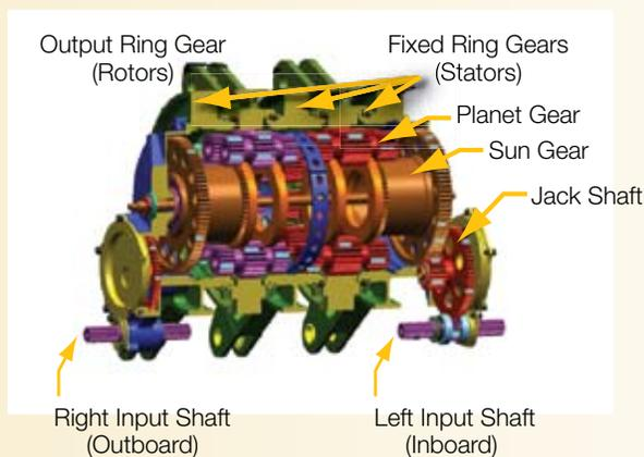
*Rudder/Speed Brake cut-away view*
