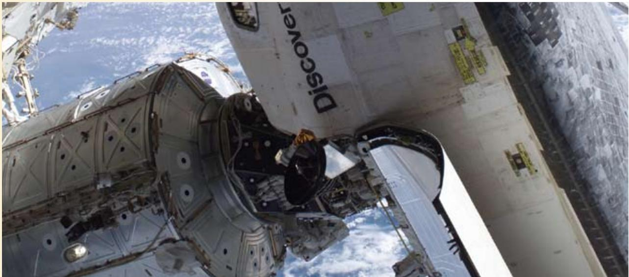
*The Space Station to Shuttle Power Transfer System will extend the amount of time an Orbiter can remain docked to the International Space Center by four to five days*
