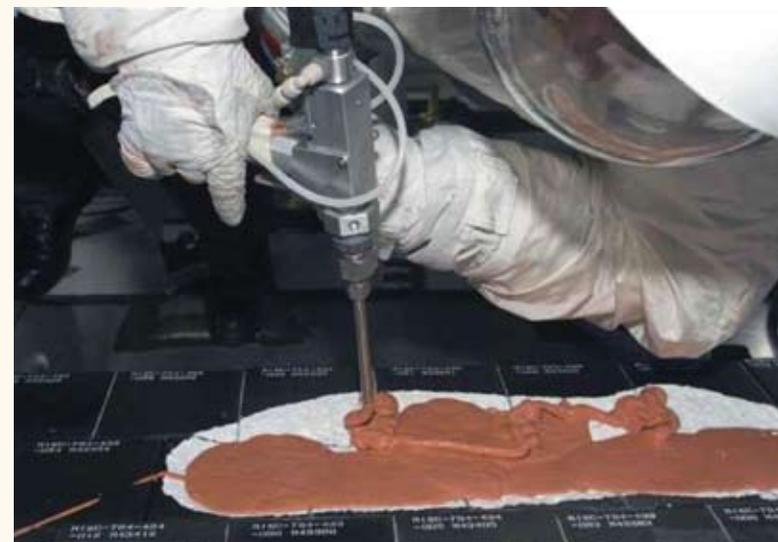
*Repairing of damaged Shuttle tiles: testing the application of STA-54 Cure-in-Place Ablative Applicator to simulated damage of the Orbiter's thermal protection tiles*
