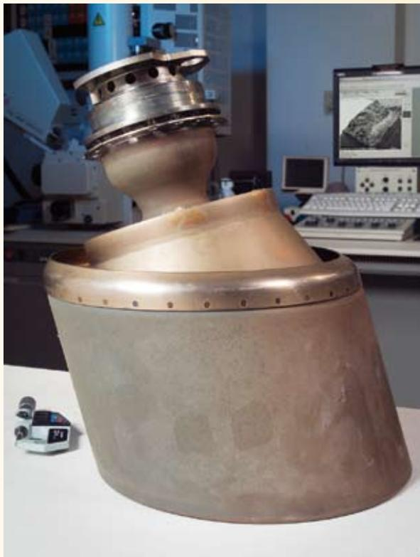
*Orbiter Reaction Control Thruster undergoing examination for cracks by the Near Field Emissions Electron Microscope in the Electron Optics Laboratory, Glenn Research Center*
