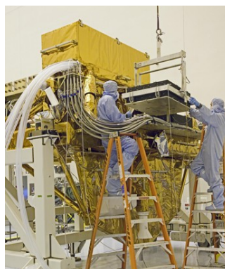
Goddard engineers install Hubble's new batteries onto the Super Lightweight Interchangeable Carrier.
