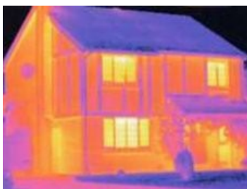
Thermographic image shows areas of high heat loss (red and yellow). Image Credit: The Insuladd Company
