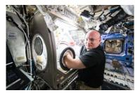
Astronaut Scott Kelly is photographed working with the Microgravity Sciences Glovebox (MSG) during a separate CASIS Rodent Research session using the Bone Densitometer Credits: NASA
