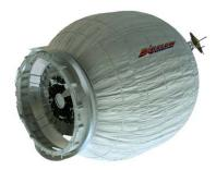
The Bigelow Expandable Activity Module (BEAM) is an experimental expandable capsule that attaches to the space station. Credits: Bigelow Aerospace, LLC
