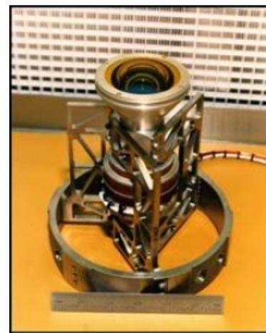
Optics in the Lightning Imaging Sensor telescope.
