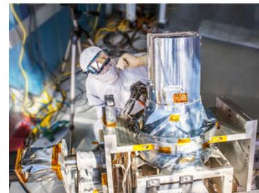
SAGE III will measure aerosols, ozone, water vapor and other gases to help scientists better understand levels of ozone in the Earth's atmosphere.
