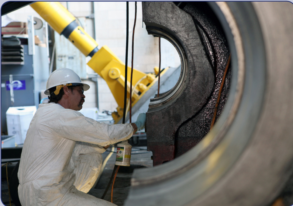
A ground support technician works on hardware in between the front of the crawler-transporter 2 (CT-2) treads in High Bay 2 inside the Vehicle Assembly Building at Kennedy Space Center on March 31, 2015. GSDO is overseeing the upgrades to the 50-year-old CT-2. New gear assemblies and jacking, equalizing and leveling (JEL) hydraulic cylinders are being installed, and other components have been upgraded to ensure the crawler's ability to handle the load of NASA's Space Launch System and Orion spacecraft on the mobile launcher as it travels to the launch pad. Photo credit: NASA/Dimitri Gerondidakis
