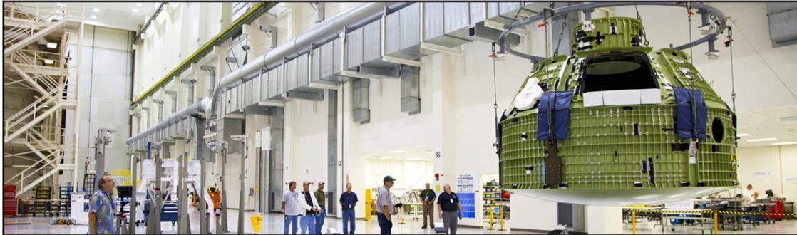
The Orion crew module is lifted onto a specialized stand so technicians can begin processing the spacecraft into a flight-ready spacecraft.
