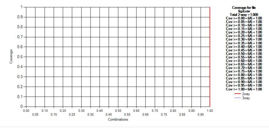
Coverage after adding test [1,0,1,0] All combinations covered to 100% level, so this is a covering array.
