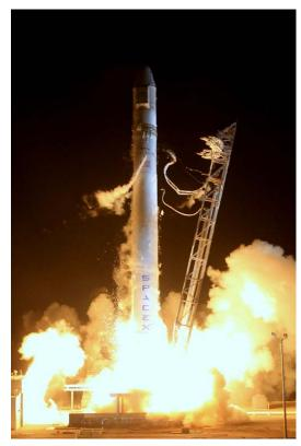
system, dubbed "Niagara," is activated. Its purpose is to suppress acoustic waves that radiate from the engine plumes, thereby mitigating the effect of vibration on the rocket. Fifty-three water nozzles set low on the launch pad provide a curtain of water flowing at 113,500 liters (30,000 gallons) a minute. The system is deactivated within 20 seconds of T-0.
