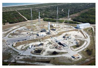
system and Dragon is mated to the rocket. The vehicle is rolled from hangar to launch pad on fixed rails shortly before launch to minimize exposure to the elements.
