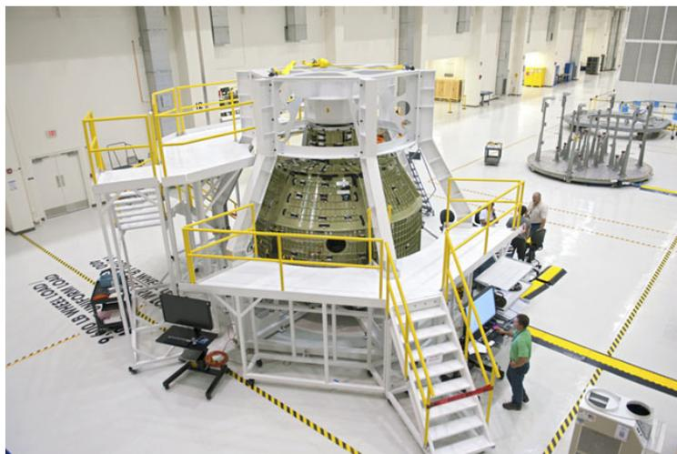
Inside the Operations and Checkout Building at NASA's Kennedy Space Center, a birdcage tool along with work platforms have been placed around the Orion Exploration Flight Test 1 crew module. The birdcage will be used to continue installation of external components in preparation for Orion's first uncrewed test flight in 2014 atop a Delta IV rocket.
