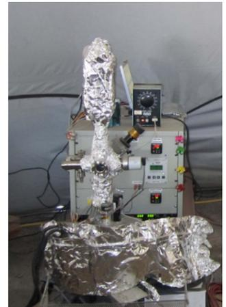
VAPoR is a miniature version of a sample analysis instrument flying on the Mars Science Laboratory. Photo credit: NASA/Danny Glavin.
