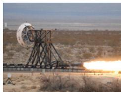
of safe landing-sites. These new devices represent the first steps on the technology pathway to land humans, habitats and return rockets safely on Mars. Flight testing is planned in fiscal year 2014 with customers that include both NASA's Mars Exploration Program and NASA's Human Exploration and Operations Mission Directorate.
