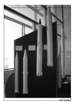
Models of several of Yangel's early missiles on display at a museum. From left to right are the R-12 IRBM (deployed 1959), the R-14 IRBM (1961), the R-16U ICBM (1963), and the original R-36 ICBM (1967). A later model of the R-36, the R-36P, was the first Soviet ICBM to be equipped with multiple independently targeted reentry vehicles.
