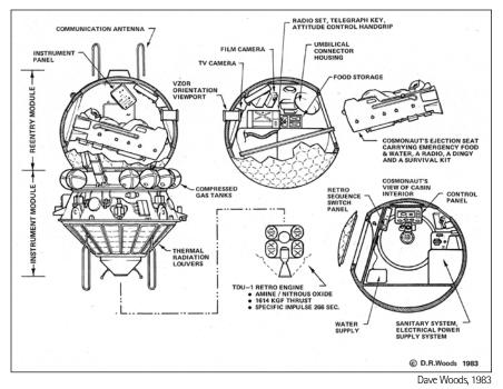
Details of the world's first piloted spacecraft, the Vostok 3KA, designed to carry a single cosmonaut into orbit.
