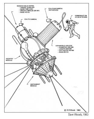
Diagram of Aleksey Leonov's historic spacewalk from *Voskhod-2* in March 1965. Note the extended airlock, which was jettisoned before reentry.
