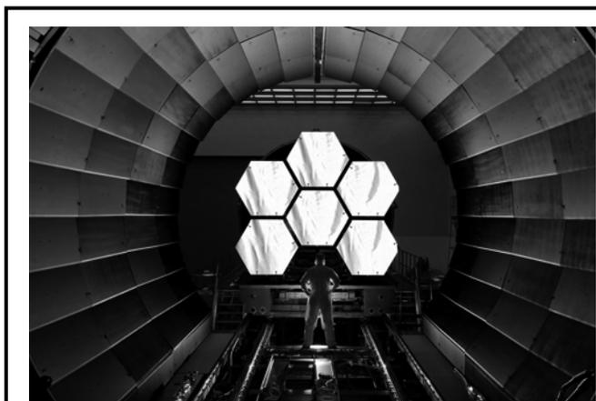
The first six flight-ready James Webb Space Telescope primary mirror segments are prepped to begin final cryogenic testing at MSFC. A total of 18 segments will form the telescope's primary mirror for space observations. Engineers began final cryogenic testing to confirm that the mirrors will respond as expected to the extreme temperatures of space prior to integration into the telescope's permanent housing structure.
