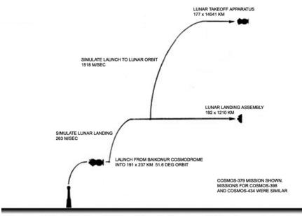
COSMOS-379 24 NOV 1970 - SIMULATE NORMAL LANDING MISSION AND RETURN TO LUNAR ORBIT USING MAIN ENGINE COSMOS-398 28 FEB 1971 - SIMULATE LANDING ABORT AND RETURN TO LUNAR ORBIT USING MAIN ENGINE COSMOS-434 12 AUG 1971 - SIMULATE NORMAL LANDING AND THEN RETURN TO LUNAR ORBIT USING BACKUP ENGINE
