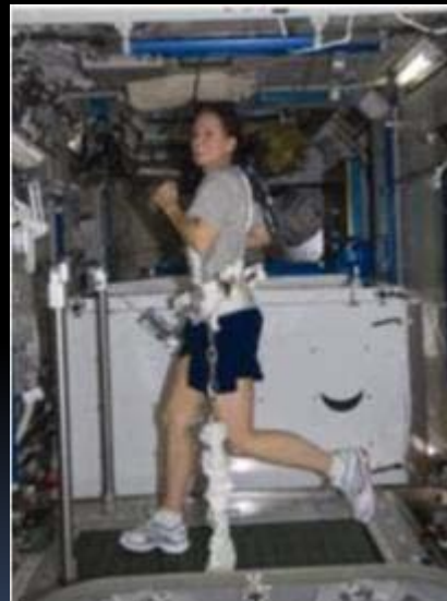
COLBERT Combined Operational Load Bearing Exercise Treadmill
