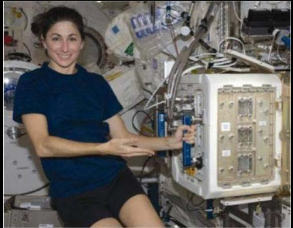
ASI Mouse Drawer System (MDS) Supported 6 mice on orbit for 90 days
