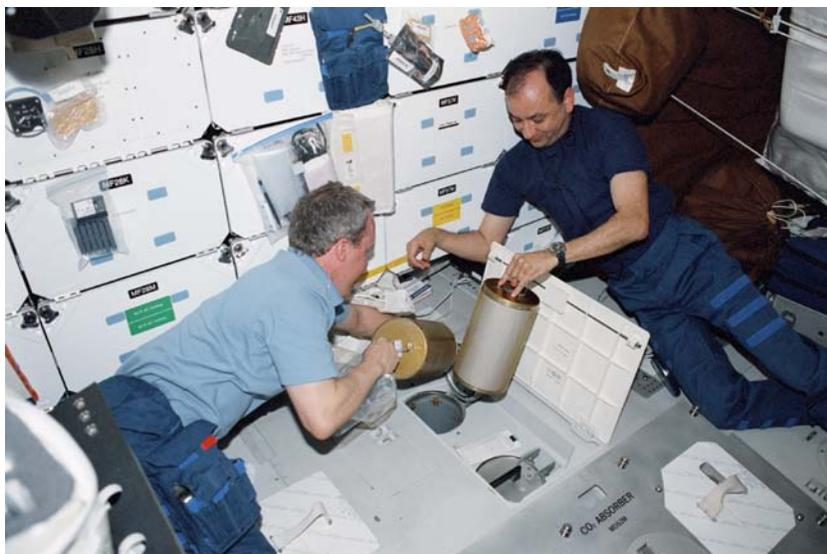
Figure 1: Astronauts Thomas D. Jones, mission specialist, and Mark L. Polansky, pilot, change out lithium hydroxide canisters on the mid deck of the Earth-orbiting Space Shuttle Atlantis.
