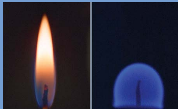
A candle flame in Earth's gravity (left) and microgravity (right) showing the difference in the processes of combustion in microgravity.
