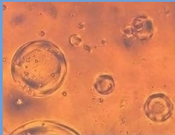
Micro-balloons containing antitumor drugs and radio-contrast oil produced in Microencapsulation Electrostatic Processing System during ISS Expedition 5.
